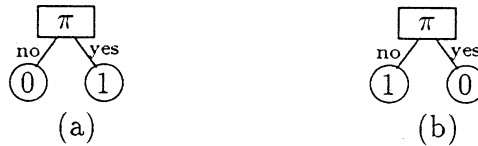
Fig. 2 A leaf is replaced by (a) or (b) for some pattern \pi .
